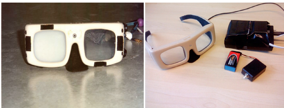
Figure 2. Plato® LC Goggles That Can Be Shut and Opened Within Milliseconds (See Left); Right: Goggles With Wireless Control
